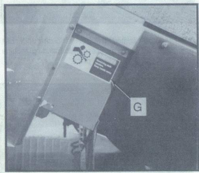
G. P/N 90162 Located on both sides of the stalk ejector drum housings to warn of hazards in the area of the rotating drums.
